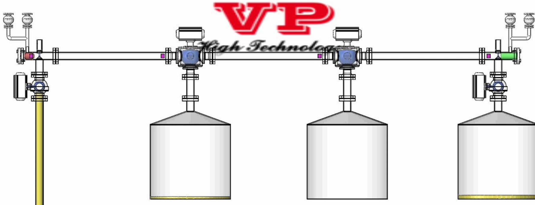
**Typical pigging system using T-Valves to deliver product to multiple tanks.**
