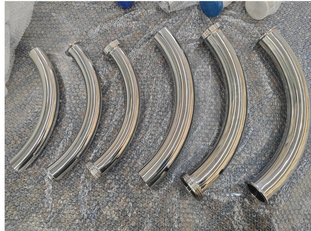
**Long Radius Elbows are necessary to ensure Pig move through smoothly in a pipping system.BJVP manufactures Long Radius Elbows in many different type of materials**
