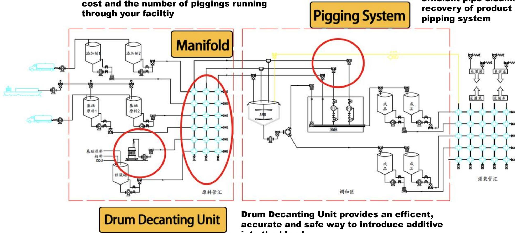
Drum Decanting Unit provides an efficient, accurate and safe way to introduce additive into the blender
